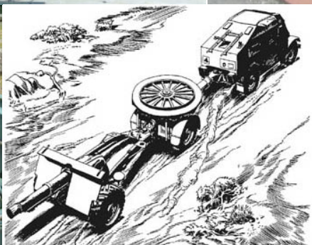
25-pounder Field Gun, showing the method by which it is transported
